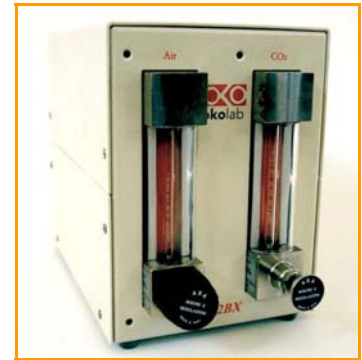
2 Gas Line Control Unit
