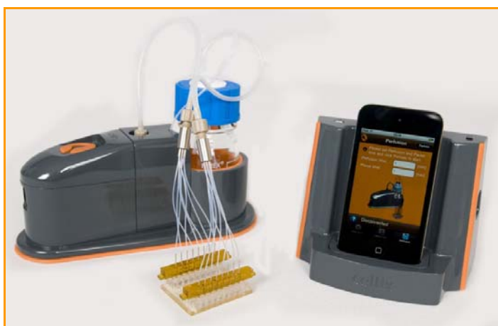
Kima Pump with iPod Touch and controller and connected via tubing to Vena8 biochip
