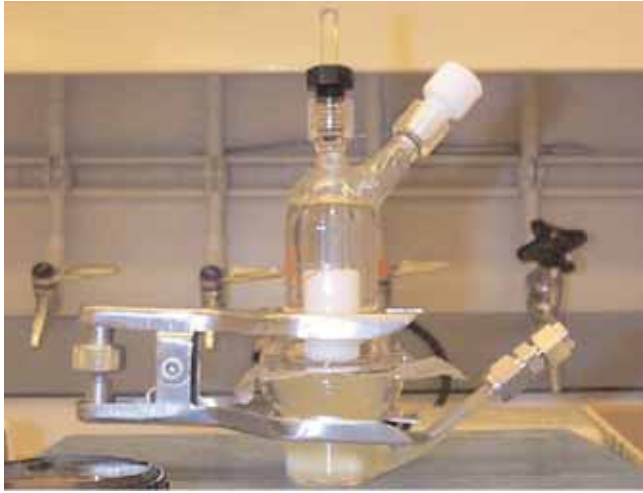
Figure C-9 Small stirred cell for transport measurements with flat sheet membranes
