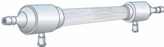
Figure A-46 Schematic of a typical tangential (cross flow) hollow fiber module
